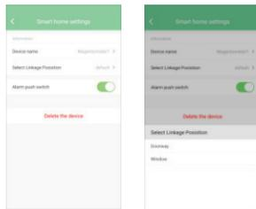
After door/window sensor or PIR are triggered, the camera will turn to the appointed position, stop for 2 seconds and take photo automatically and save into Message --- Smart Home Equipment (see the red remark eg5.4), finally turn to the quandam position, meanwhile, on mobile APP, it will show hint message.
